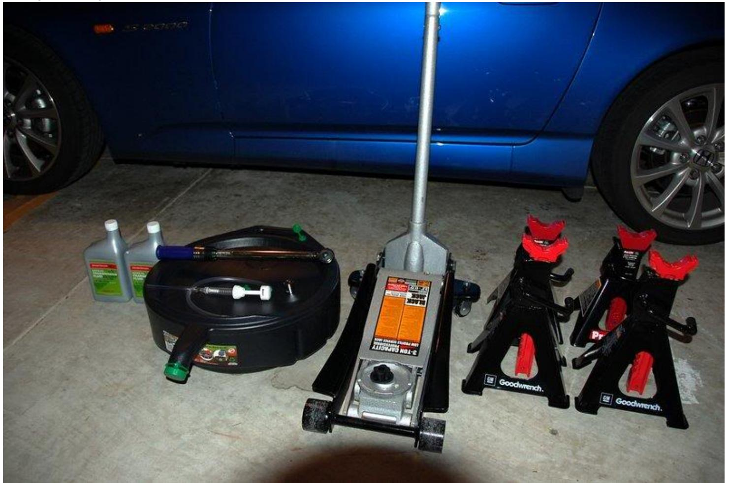
I use 4 jack stands in order to keep the car level so that I don't have to lower it and raise it back up to drain. You can use two jack stands to raise only the front, but you'll want to lower the car while it is draining to ensure complete drainage, and again after filling but before replacing the fill bolt to allow the fluid to drain to the proper level.
