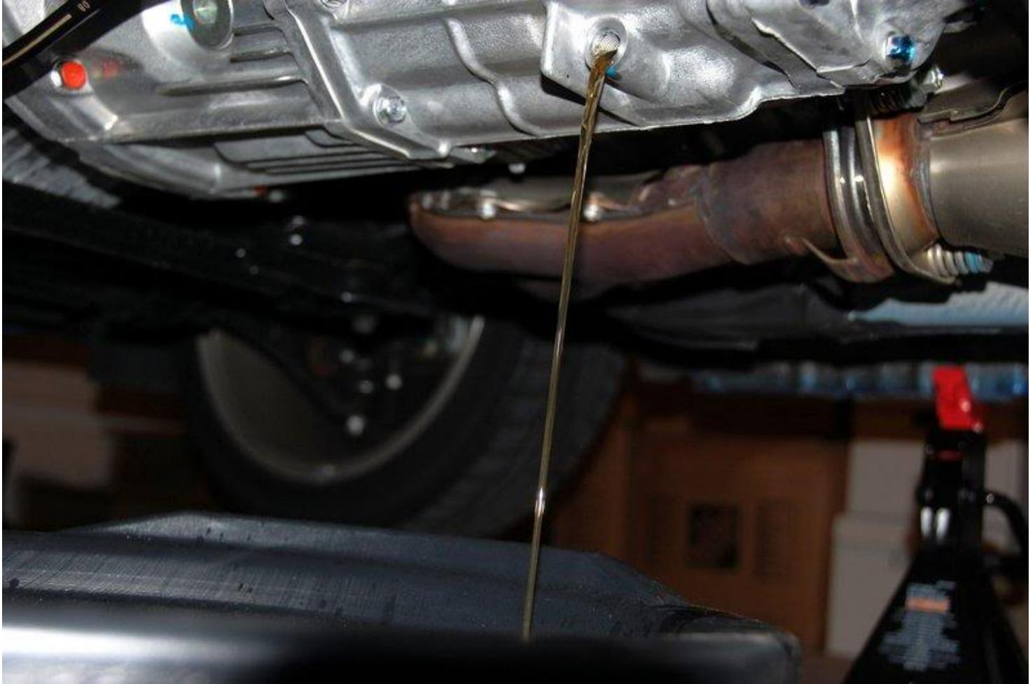
Allow the transmission to drain completely. At this time you can clean off your fill and drain bolts and put the new washers on them. Be sure to position the washers so that the flat side will be towards the transmission.
