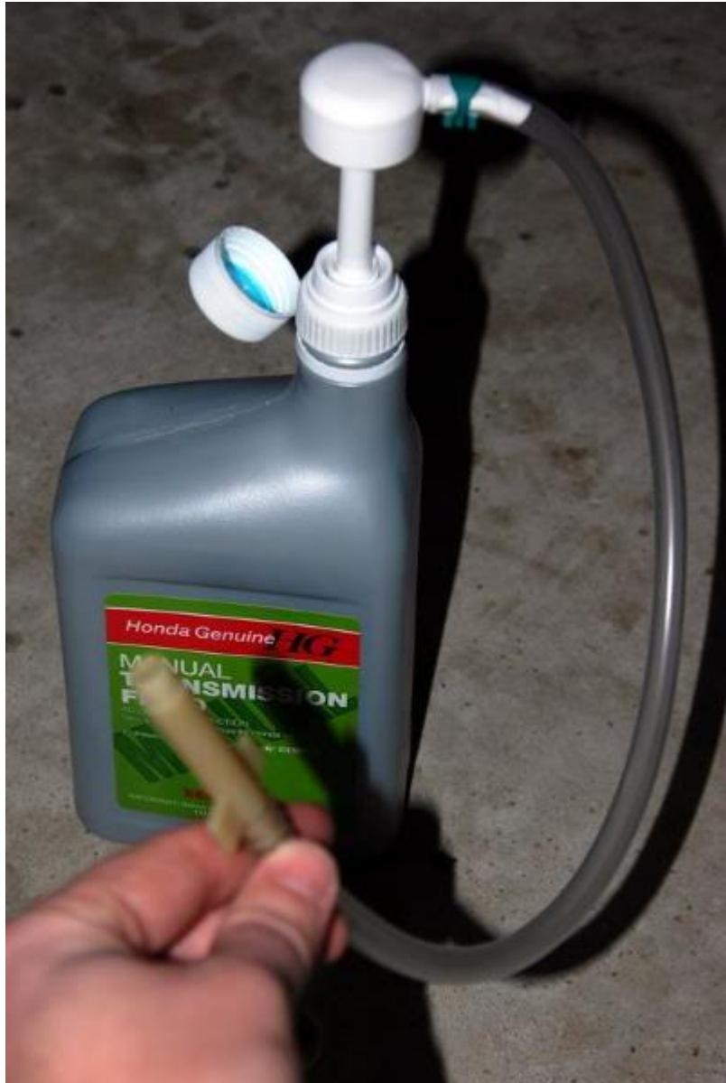
After pumping in a little new fluid and allowing it to drain completely, screw the drain plug back in using your torque wrench and tighten to 29 lb-ft. Now pump your new tranny fluid into the case until it begins to run out the hole.
