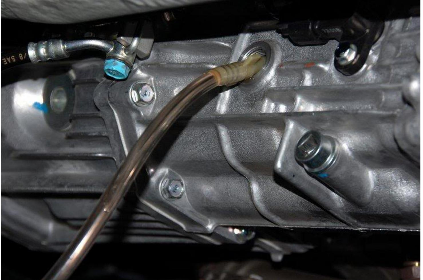
When it starts running out of the hole, use your torque wrench to screw the fill plug in and tighten to 33 lb-ft. Use rags or paper towels to clean up the outside of the case and you're done! Lower your car and hop in. You should be able to feel the transmission shifting more smoothly. Take it for a casual drive to make sure everything works properly. If so, have a cold one and celebrate all the money you saved and rest easy knowing everything was done right.
